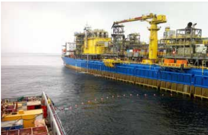
Nitrogen Injection in progress with buoys attached to the hose
