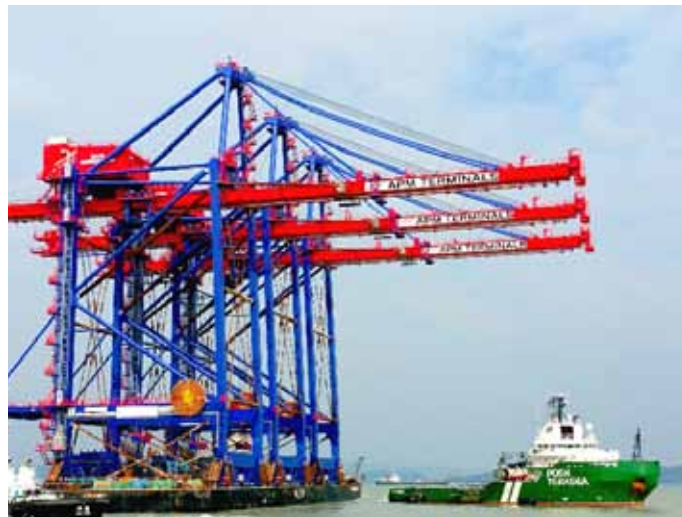
12,000BHP 150TBP AHT Salvigilant towing POSH Giant 1 loaded with three STS cranes out of Zhangzhou, China
