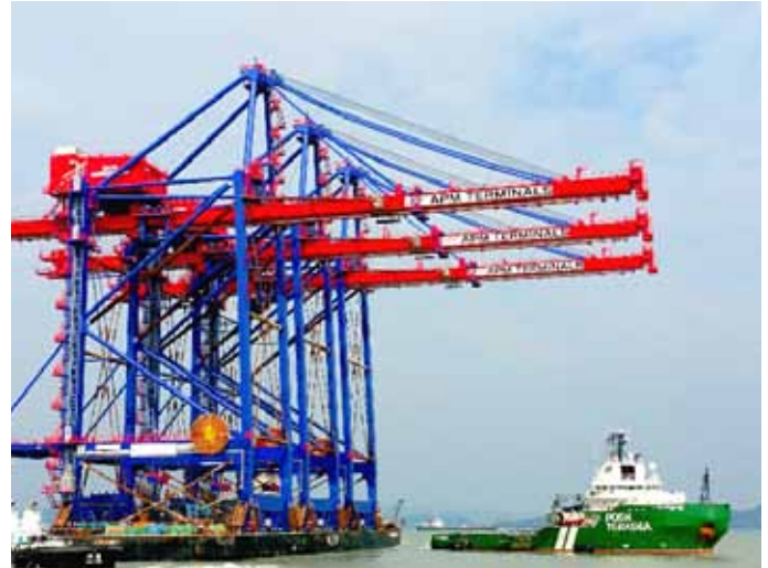
12,000BHP 150TP AHT Salvigilant towing POSH Giant 1 loaded with three STS cranes out of Zhangzhou, China
